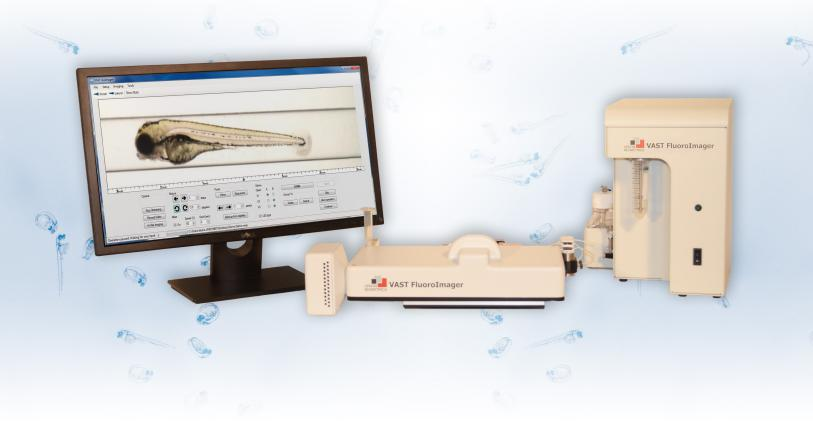
**The VAST FluoroImager** automates positioning of 2-7 dpf zebrafish larvae. The larvae are oriented accurately and reproducibly within a glass capillary using a set of rotational motors.
