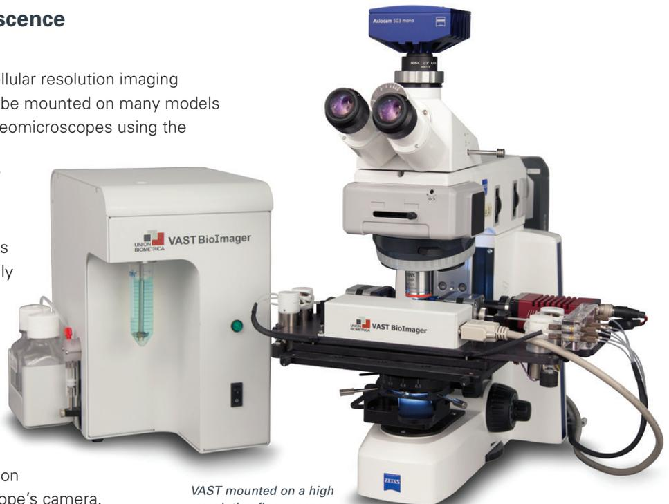
VAST mounted on a high resolution fluorescence microscope
