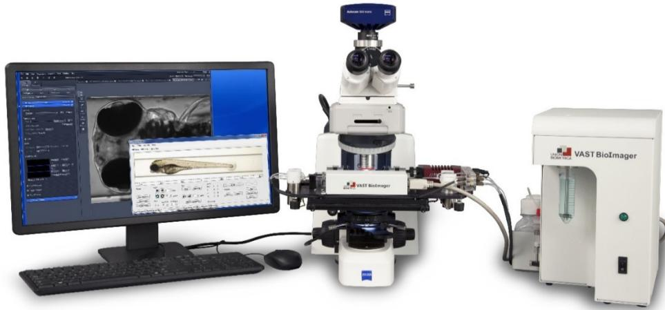
**Figure 1.** VAST BioImager mounted on high-resolution compound microscope for automated positioning and imaging of zebrafish larvae.
