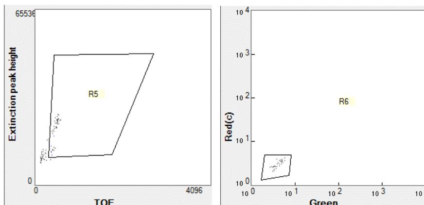
**Figure 2:** Negative control sample. Plots show the size (TOF) and optical density (EXT) (left panel), total auto-fluorescence (Green versus Red) (right panel) of the clusters.
