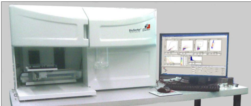
**Figure 1.** The BioSorter is a large particle flow cytometer that allows high-throughput analysis and sorting of objects in the size range 10  $\mu\text{m}$  to 1500  $\mu\text{m}$ .
