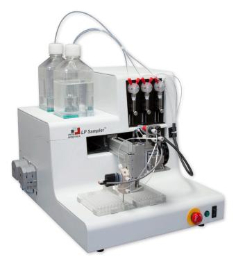
The Large Particle Sampler (LP Sampler<sup>™</sup>) module is the only automated sample introduction system designed specifically for gentle handling of large, fragile objects such as
