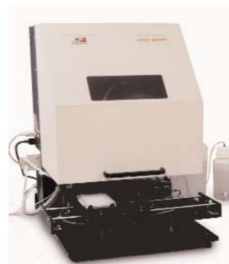
**Figure 1.** The COPAS *PLUS* was used to dispense *Arabidopsis* seeds in a microtiter format in less than 2 minutes.
