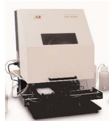
Figure 1. The COPAS BIOSORT® was used to sort C.elegans into 96 well microtiter plates.
