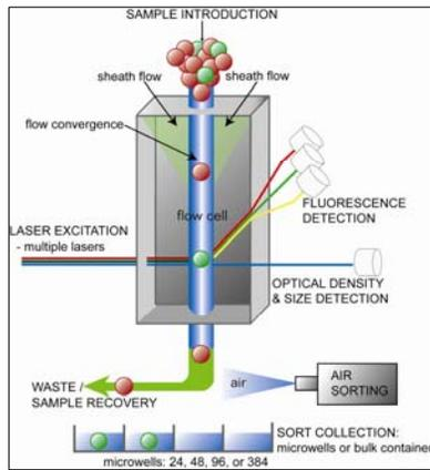
**Figure 1:** BioSorter analyzes and sorts cell clusters and large cells (1-1500 µm diameter) in a continuous flow stream at high rate (up to 100 ev/sec). The device measures object size (TOF), optical density (EXT) and multiple fluorescent markers.
