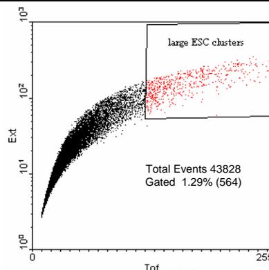
Figure 2. Parameters for isolating hESC clusters. Time of flight (TOF) is the proxy measurement for the size, reflected by the time that it takes the object to pass through 670nm red laser beam. Single cells and ESC clusters can all trigger the registration of an event; large ESC clusters (>20 cells/cluster) differ from single cells and small clusters in their large TOF and EXT values. We examined the sorted clusters by microscopy to optimize sorting parameters.
