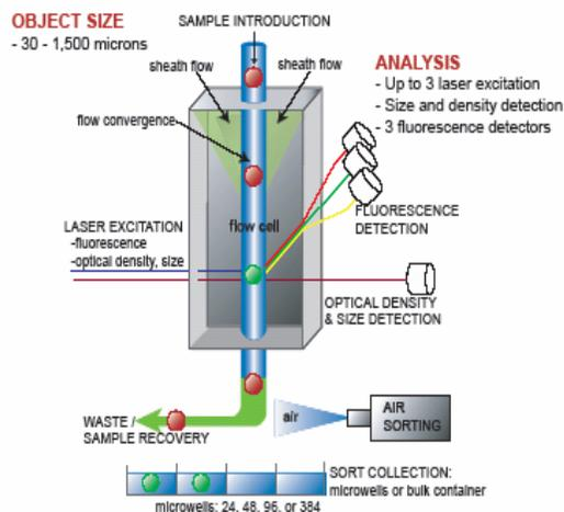
Figure 1. Schematic diagram of fluidics, optics & sorting mechanism. Key features of COPAS BioSorter include:
