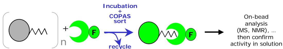
Beads in a library that have bound to a fluorescently labelled target protein can be sorted in a matter of minutes from the bulk of beads that do not bind to the target. (see also figure 1) By setting differential sort parameters, it is possible to sort strong from weak
