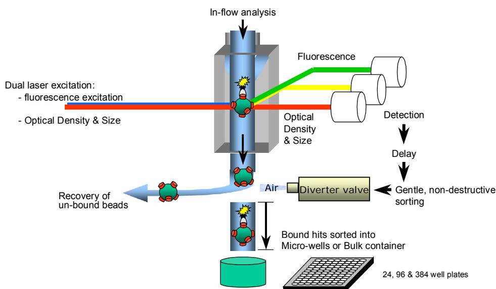
Figure 3: Schematic of **COPAS** flow sorting
