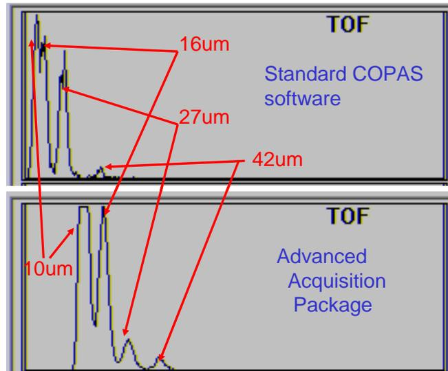
Figure above illustrates improved resolution between 10 $\mu$  and 16 $\mu$  particles by using AAP.
